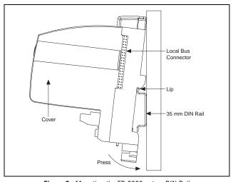
$\textbf{Figure 2.} \ \ \text{Mounting the FP-3000 onto a DIN Rail}$
